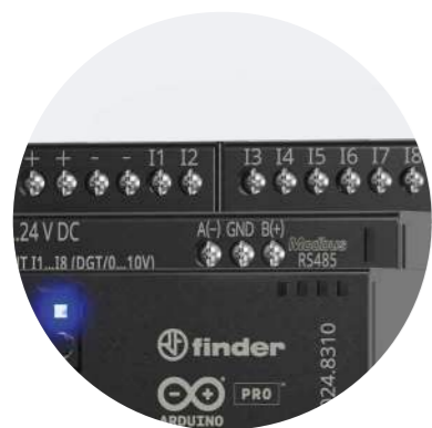
8 inputs and 4 outputs
